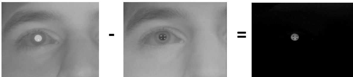
FIGURE XXIV Example of final data provided by updated hardware setup. The dark pupil image is subtracted from the bright pupil image to remove ambient noise. Only the actual signal, the pupil and glints, remains.
