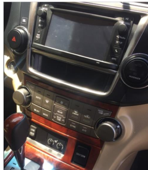
Figure 3. 2013 Toyota Highlander Limited infotainment system with Toyota Extension Box.
