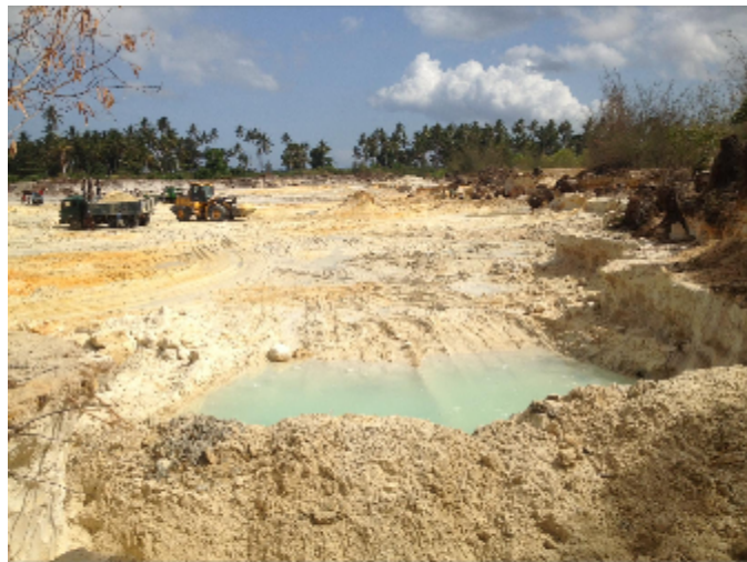
Figure 10 : The Chechele site at Donge, an example of groundwater intrusion into the quarry.
