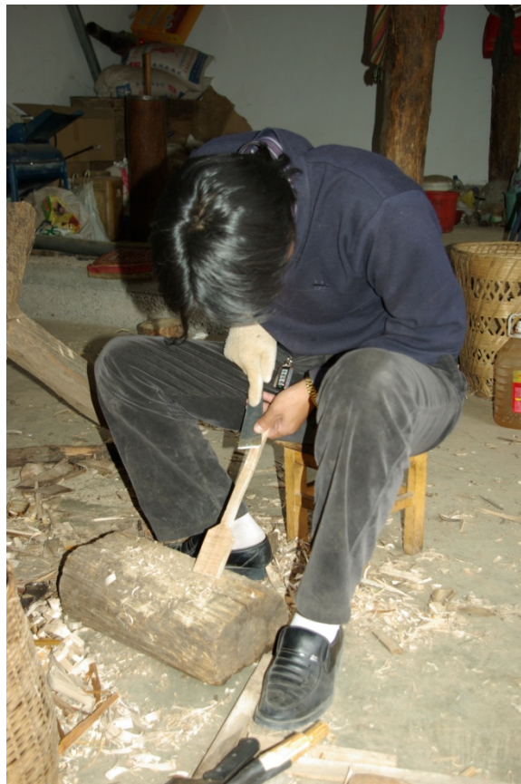
Figure 12: A chisel is used to thin and smooth the handle of a paddle.
