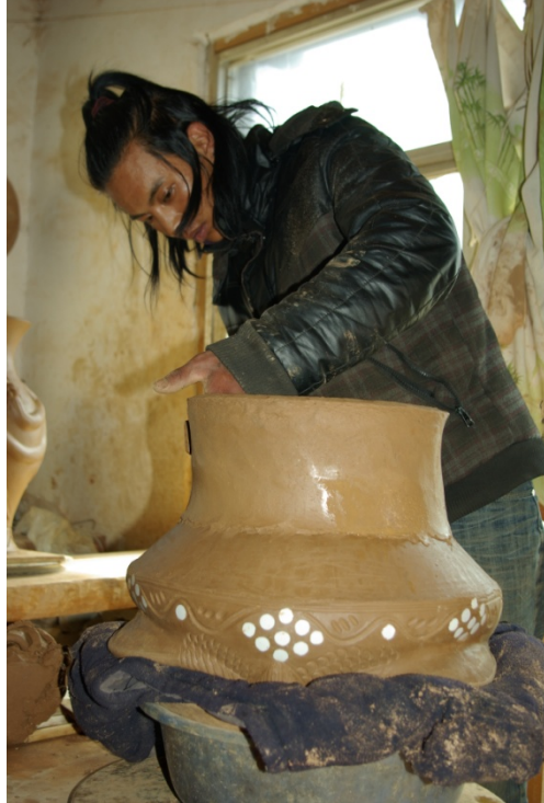
Figure 7: A potter seals the seam of a slab recently attached to the rounded base of a firepot.
