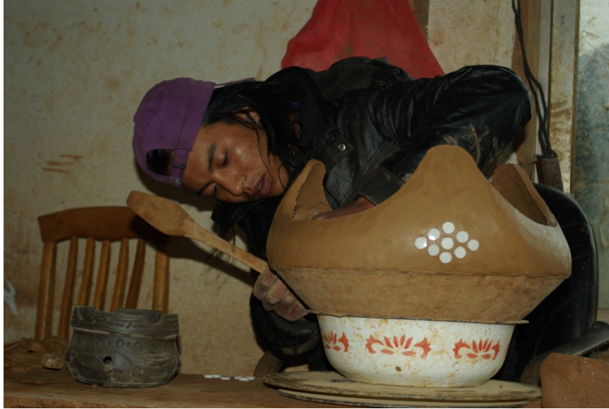
Figure 11: A potter porcelain pieces into the clay while supporting the form from the inside.
