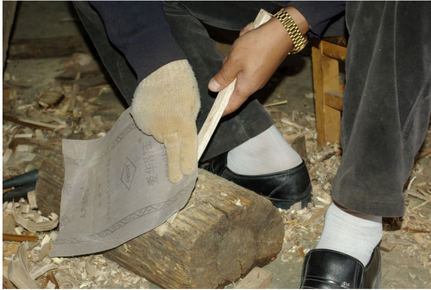
Figure 13: Sandpaper gives wooden tools their smoothness.
