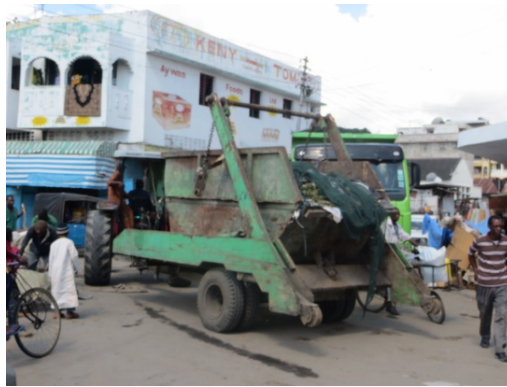
Figure 6: Bulk container trailer
