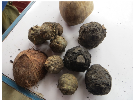
F1: “Waste” charcoal from materials like paper, coconut shells, leaves, maize cob, clay and charcoal ash.
