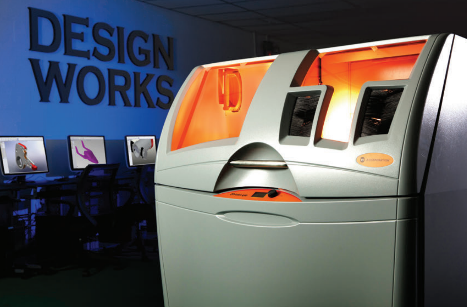
RCBI's Z Corp. 450 3-D printer creates full-color objects by combining a dust-like resin powder with inks and a bonding agent. Like other 3-D printers, the ZPrinter can produce moveable objects that require no assembly.
