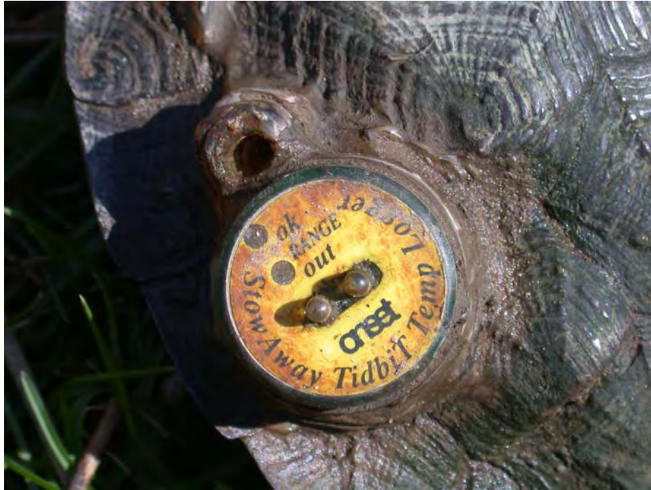
FIGURE 3.7. A CLOSE-UP OF A DATALOGGER ATTACHED TO A WOOD TURTLE. PHOTOGRAPH BY ARIANA N. BREISCH 2001.
