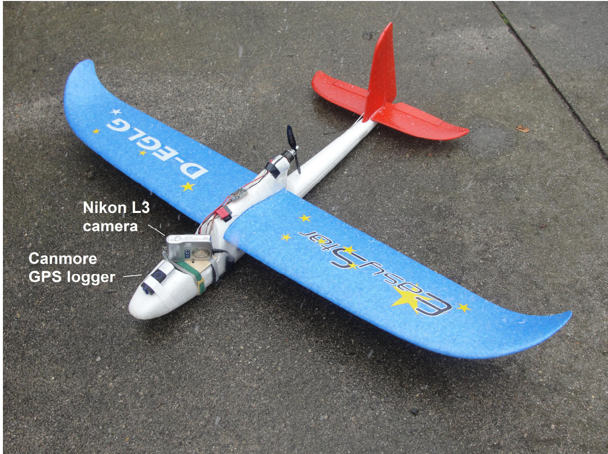
Plate 1. Multiplex Easystar with Nikon L3 rigged for taking oblique photos.
