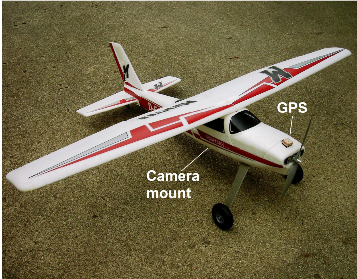
Plate 2. Multiplex Mentor. GPS antenna is directly behind propeller.
