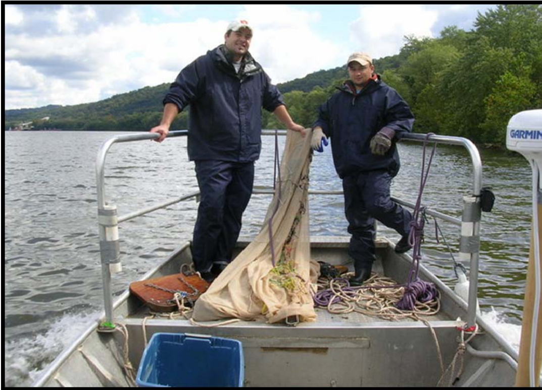
Figure 19. Eight foot wide Missouri modified benthic trawl on the front of the electrofishing boat ready to be deployed
