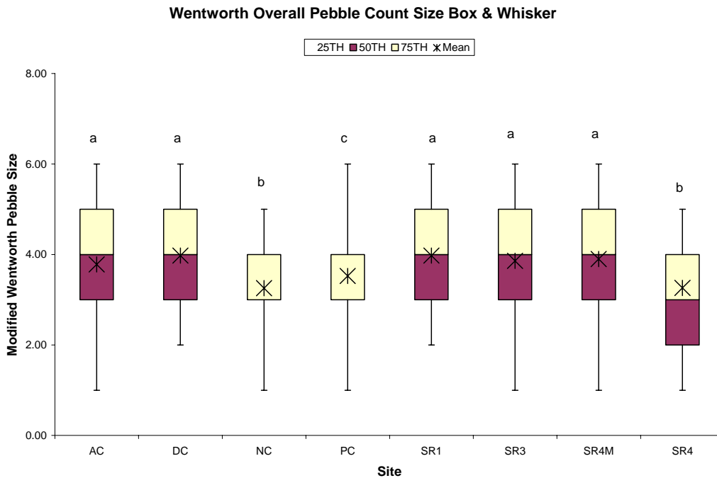
Figure 4.4. Box and Whisker Plot of Overall Modified Wentworth Pebble Count Data (Boxes with the same letter are not significantly different as determined using Student-Newman-Keuls ( \alpha = 0.05 ); see Table 3.2 for pebble count sizes)
