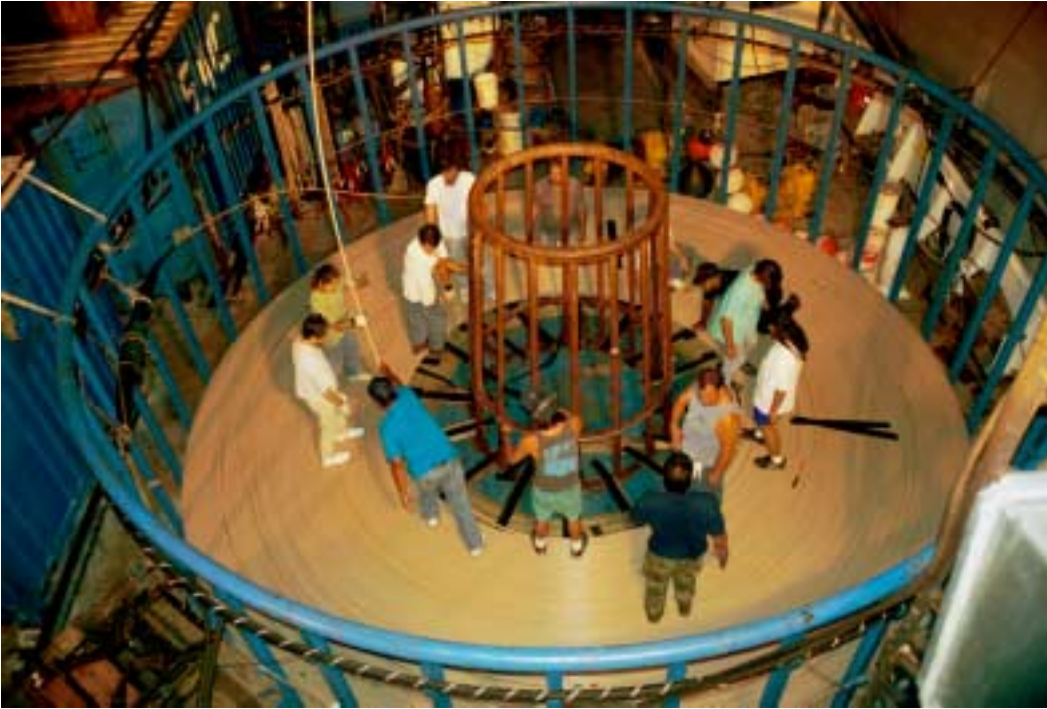
Figure 6. Loading the HUGO cable on the R/V Independence. 24 hours were required to load 47 km of cable.
