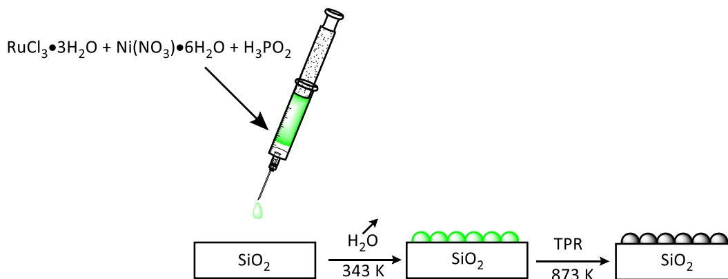
Figure 2.1: Process for Ni x Ru 2-x P/SiO 2 catalyst synthesis.
