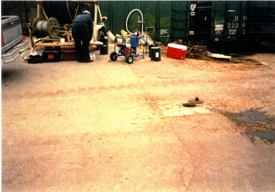
Photo 5. Waterra Groundwater Sampling Pump (in place over well P-3). Well P-3D in foreground.
