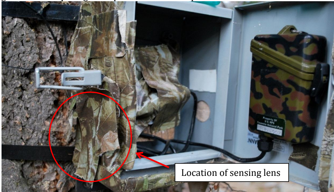
Figure 20: In this tampering example camouflage tape from the counter's casing was placed over the lens.
