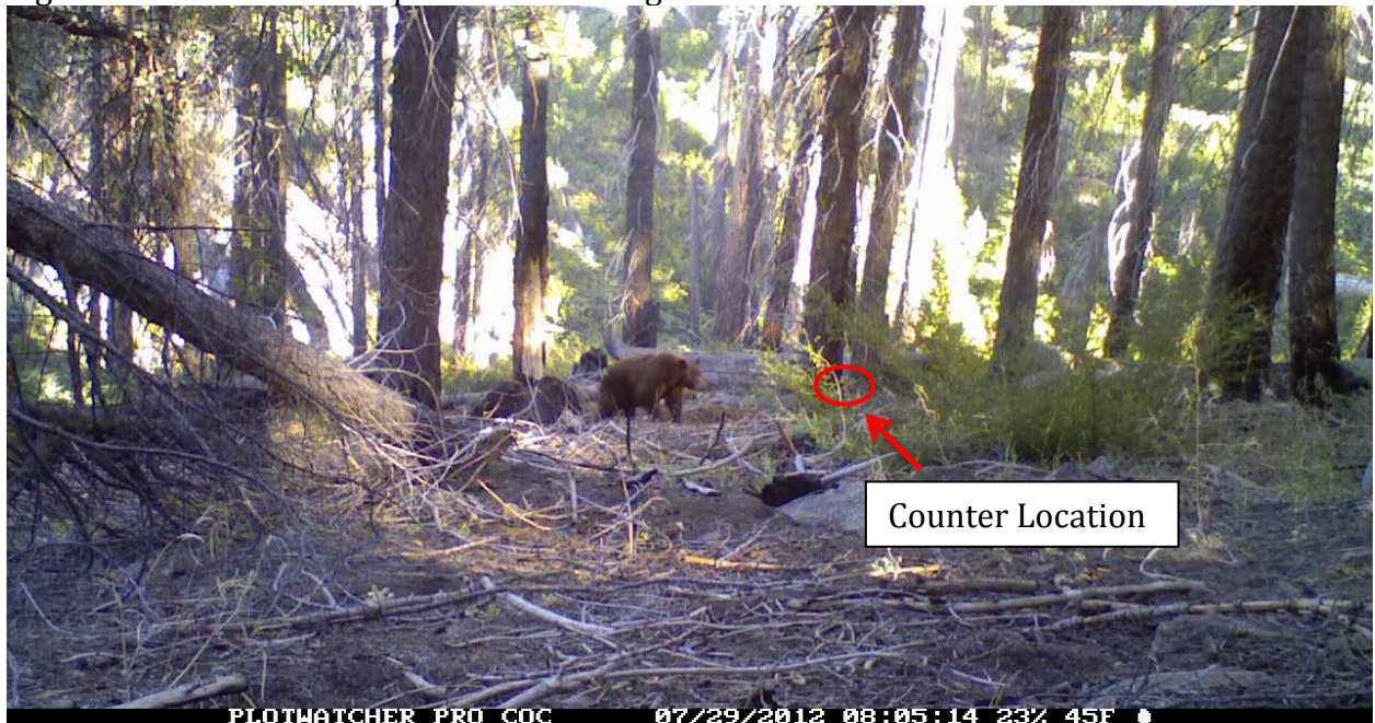
Figure 8: In this figure a miscount occurs on a low use trail when a bear passes the infrared trail counter and registers as an event.
