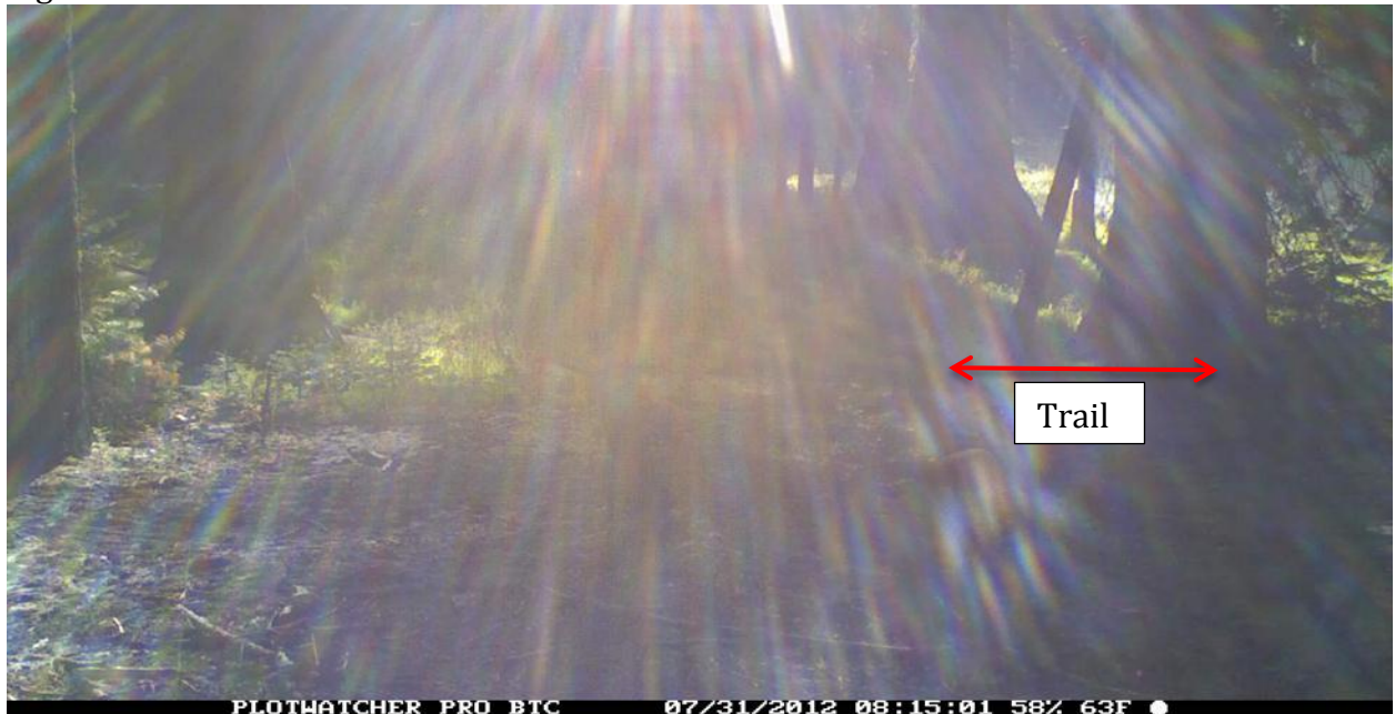
Figure 23: In this example poor placement of the time-lapse camera results in the morning sun blinding the lens.
