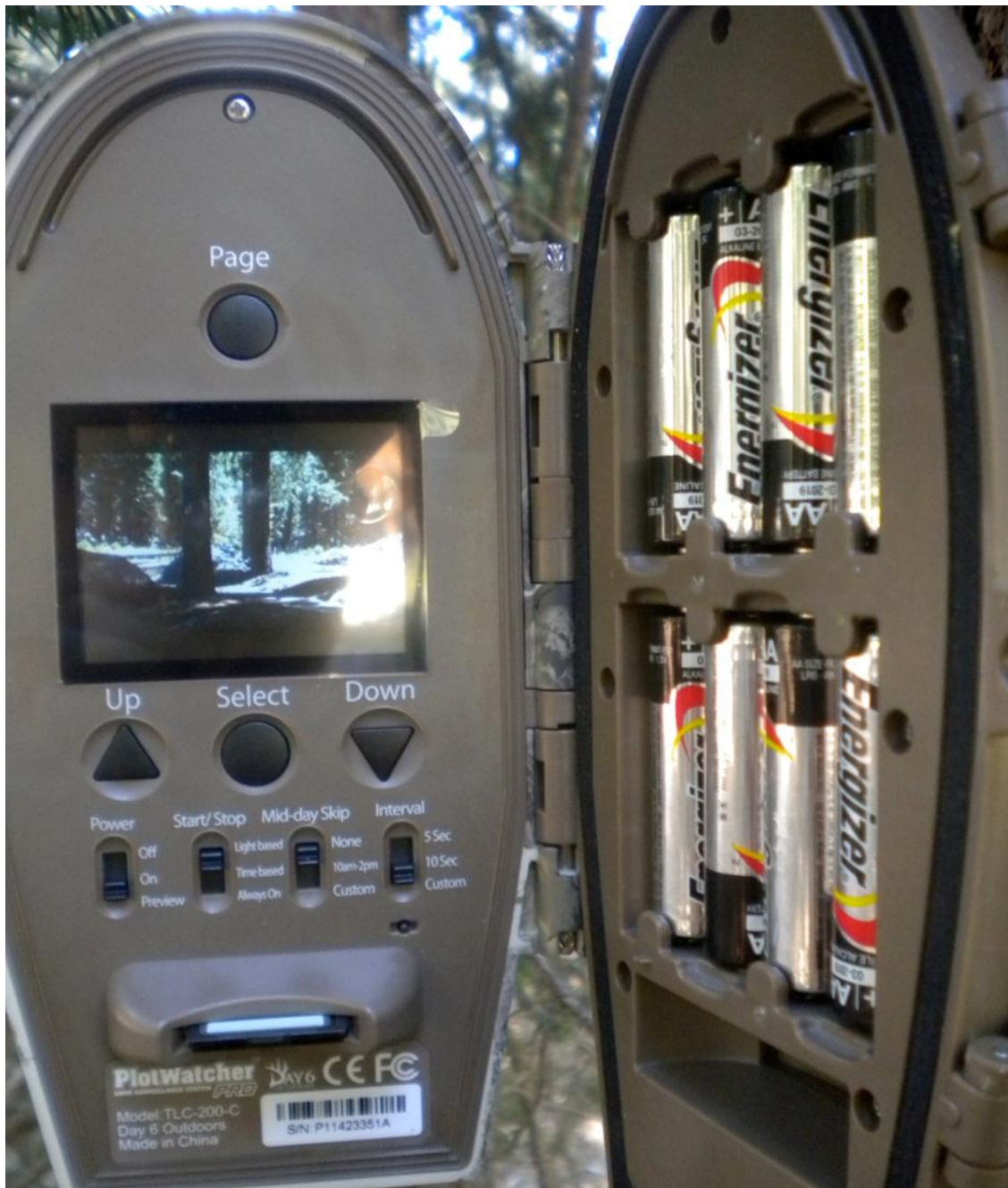
Figure 14: Powered by eight AA batteries, the PlotWatcher Pro comes with a variety of formatting options. Able to preview the location of the camera shot, data is recorded on micro SD cards, which were then transferred to a computer for analysis.
