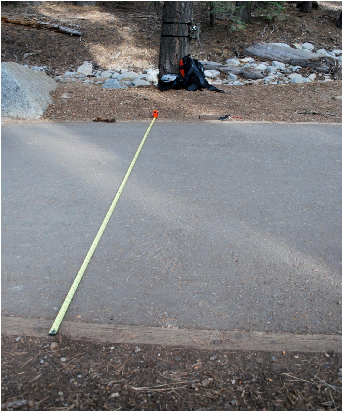
Figure 28: At each trail, width was measured by placing a measuring tape flat across the area seeing most traffic.
