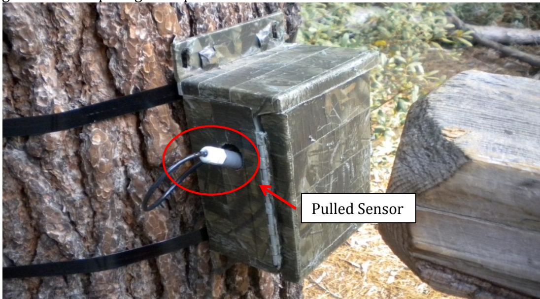
Figure 21: In this tampering example, the counter's infrared counting scope was pulled from the box then jammed back in.
