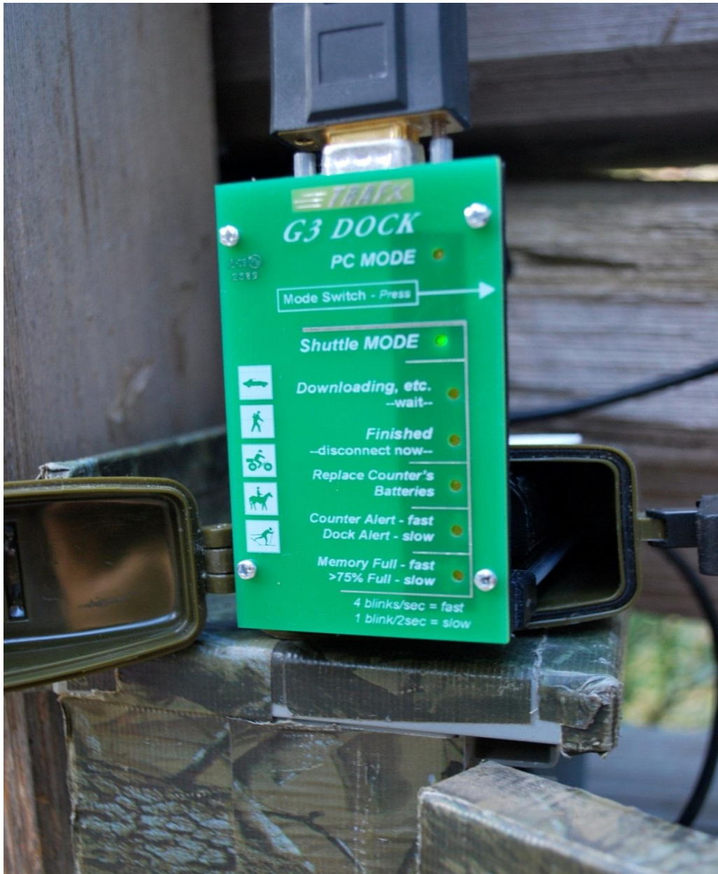
Figure 12: The TRAFx G3 Dock was used to hold and transport counter data from the field for later analysis. Connecting easily with the TRAFx trail counter, this device was used for quick extraction without bringing attention to the counter's locations. Once data were obtained transfer to a computer was done seamlessly, requiring only a quick reformatting from text file to an Excel spreadsheet.
