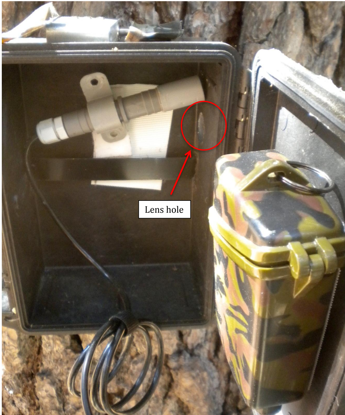
Figure 22: In this example the infrared trail counter lens has been punctured, then shoved back into the protective box casing.
