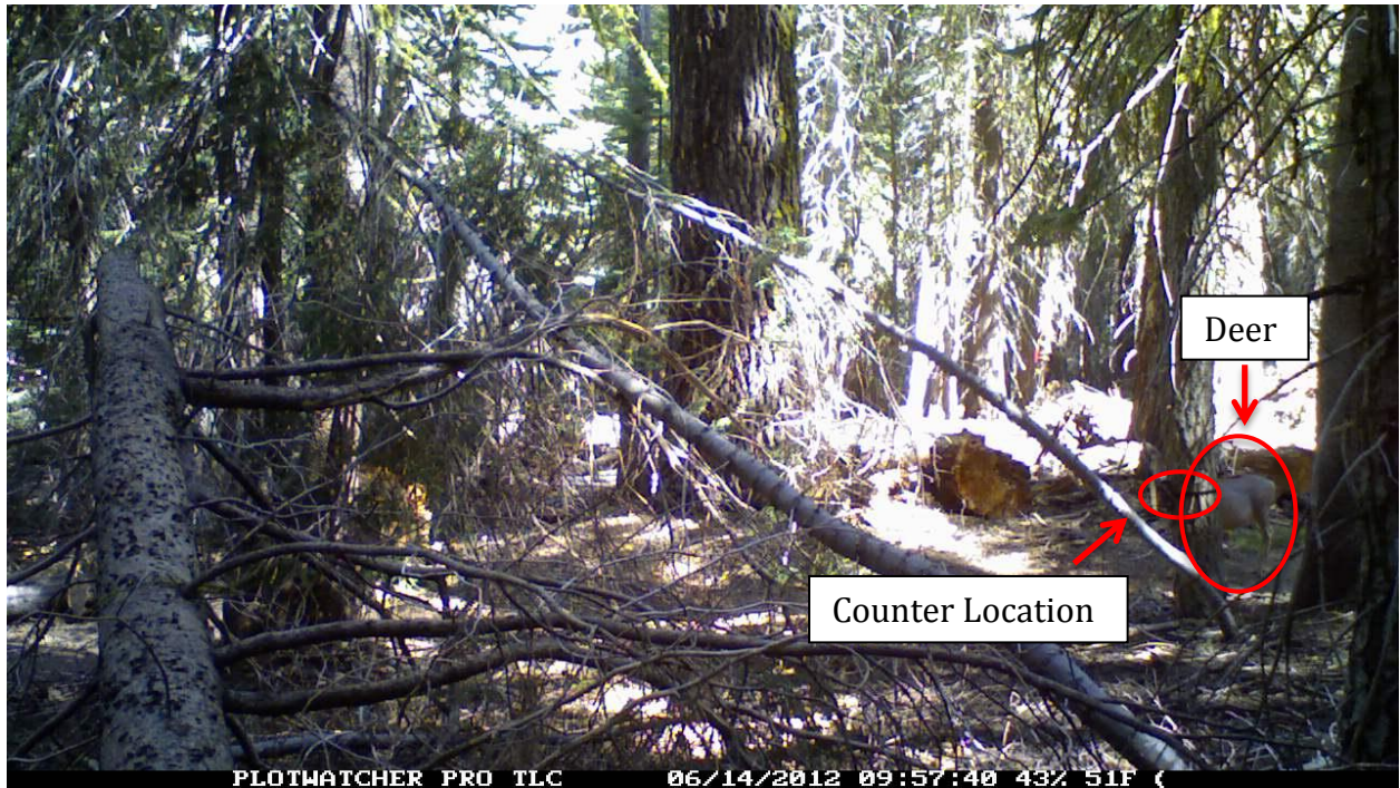
Figure 9: In this example miscount occurs when a curious deer stops to examine the trail counter and consequently causes multiple false events to be registered.
