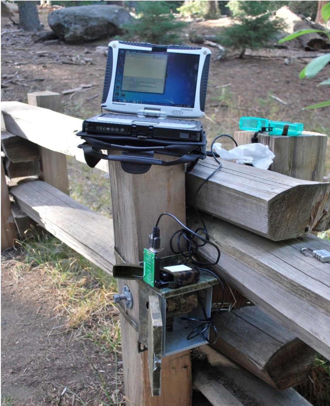
Figure 30: In this figure the download process of trail counts is demonstrated using the TRAFx infrared trail counter, the TRAFx shuttle, and a field computer.
