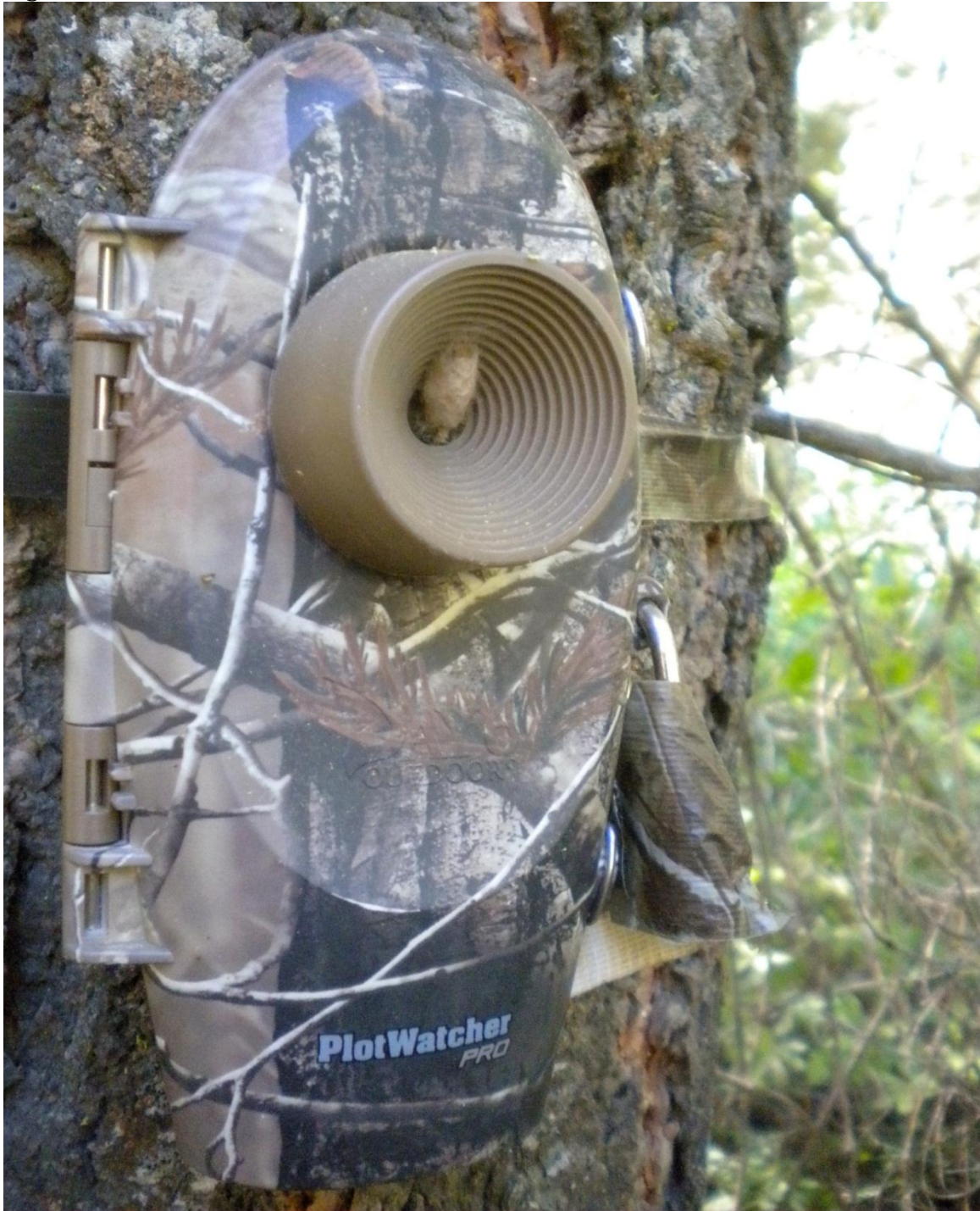
Figure 25: At this site the calibration process was set back due to a caterpillar making its cocoon directly over the lens.
