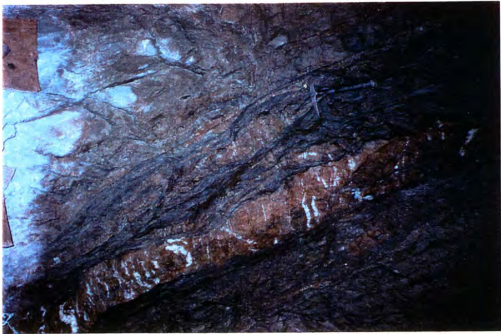
Figure 9a. Face photo from 3700 ER2B E showing several features of the West Chance vein system as referred in text. Quartz ladder veins in siderite veins, anastomosing nature of shears, fractures, and veins; comparison of splays and Riedel shears; and cross-cutting relationships between extension veins and discharge veins.
