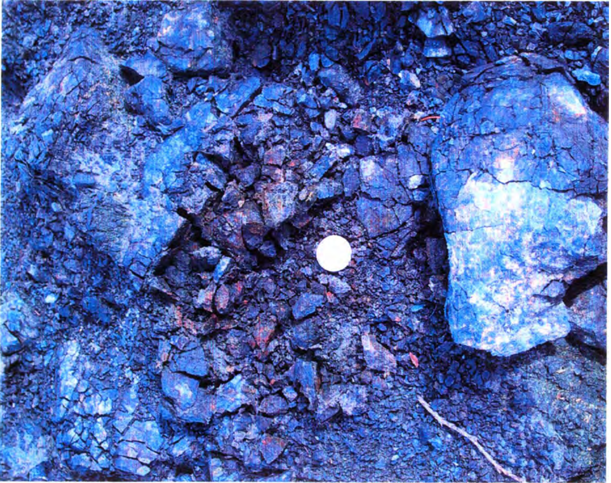
Figure 14. Serpentinitic boulder displaying in-situ disintegration.
