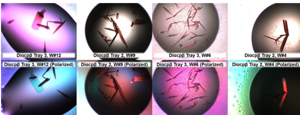
Figure 42. Examples of dia-cp \beta crystals under normal light (top) and polarized light with a cross polarized filter (bottom). Brighter sections in the polarized images are caused by higher birefringence which indicated greater order of the crystal.
