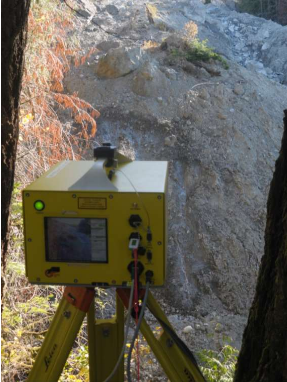
Figure 10 - The Optech ILRIS 3D laser scanner from a position on the north side of the landslide ( October, 2009).
