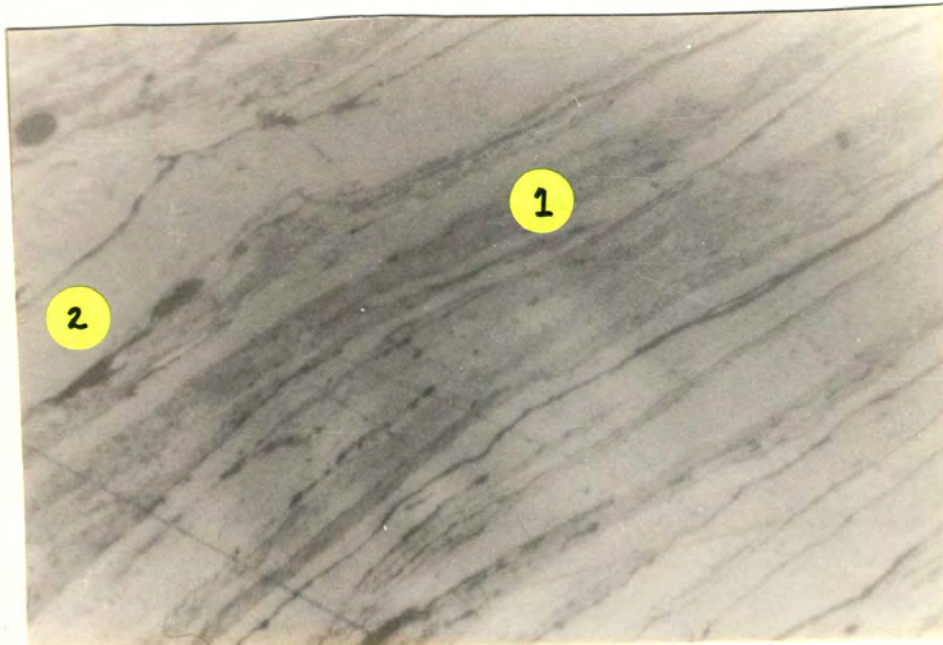
Figure 29. Diffuse clay layers (1) of variable width in vitrinite (2). Polished surface, oil immersion, x500.
