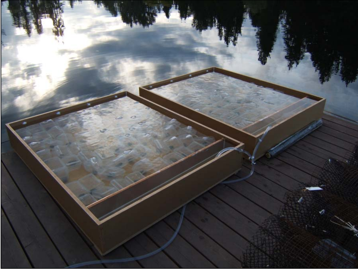
Figure 6. Continuous flow-through water tables (1.2 x 1.5 x 0.2 m each) used to hold crayfishes when not being used in field experiments at Pine Lake, Sammamish, Washington.
