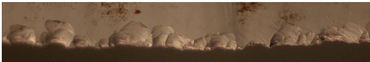
Figure 11. Example of scalar and step combination scar pattern (SCST) (45WH55-#1817).
