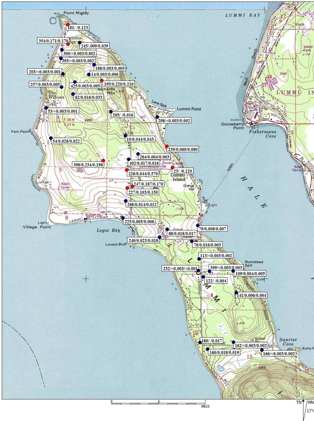
Figure 10. Well location map with arsenic concentrations for April and August sampling seasons. The wells are labeled as: well number/April arsenic concentration/August arsenic concentration. Wells marked with red symbols had an arsenic concentration greater than 0.070 mg/L for at least one sampling season. Wells with blue symbols had arsenic concentrations below 0.070 mg/L for both sampling seasons.
