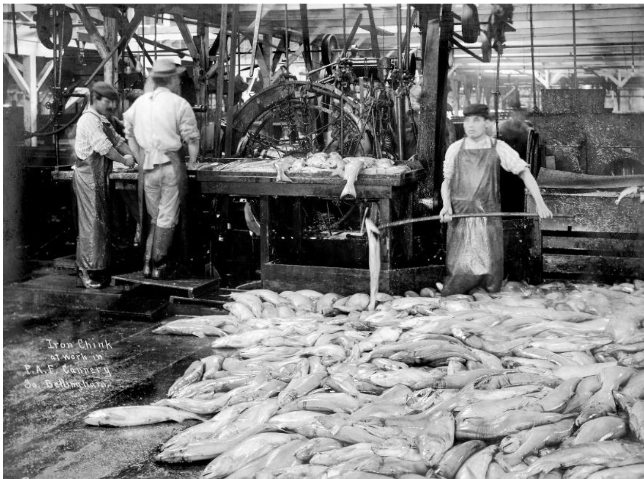
Figure 22: Iron Chink at Pacific American Fisheries receiving fish from the floor, 1906. Used with permission from the Whatcom Museum Photo Archives.
