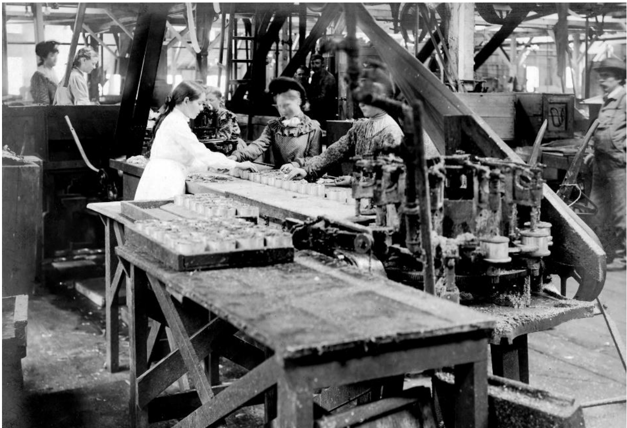
Figure 27: Woman working in line at Pacific American Fisheries, chipping and topping cans, 1906. Used with permission from the Whatcom Museum Photo Archives.
