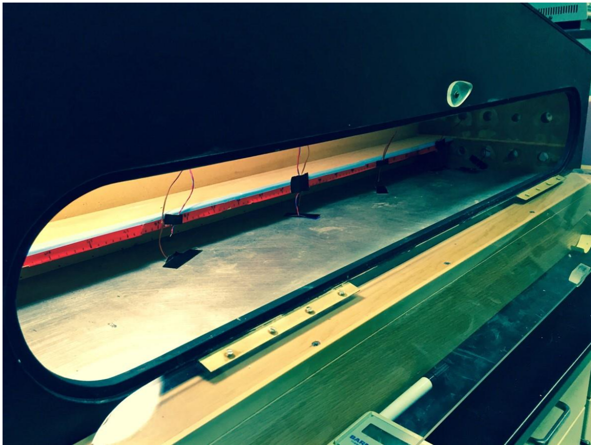
Photo 9-10. Pictured are (from top to bottom) 1) the thermal gradient (center), including the ethylene glycol cooling pump (right) and heating coil device (left), and 2) the interior of the thermal gradient.
