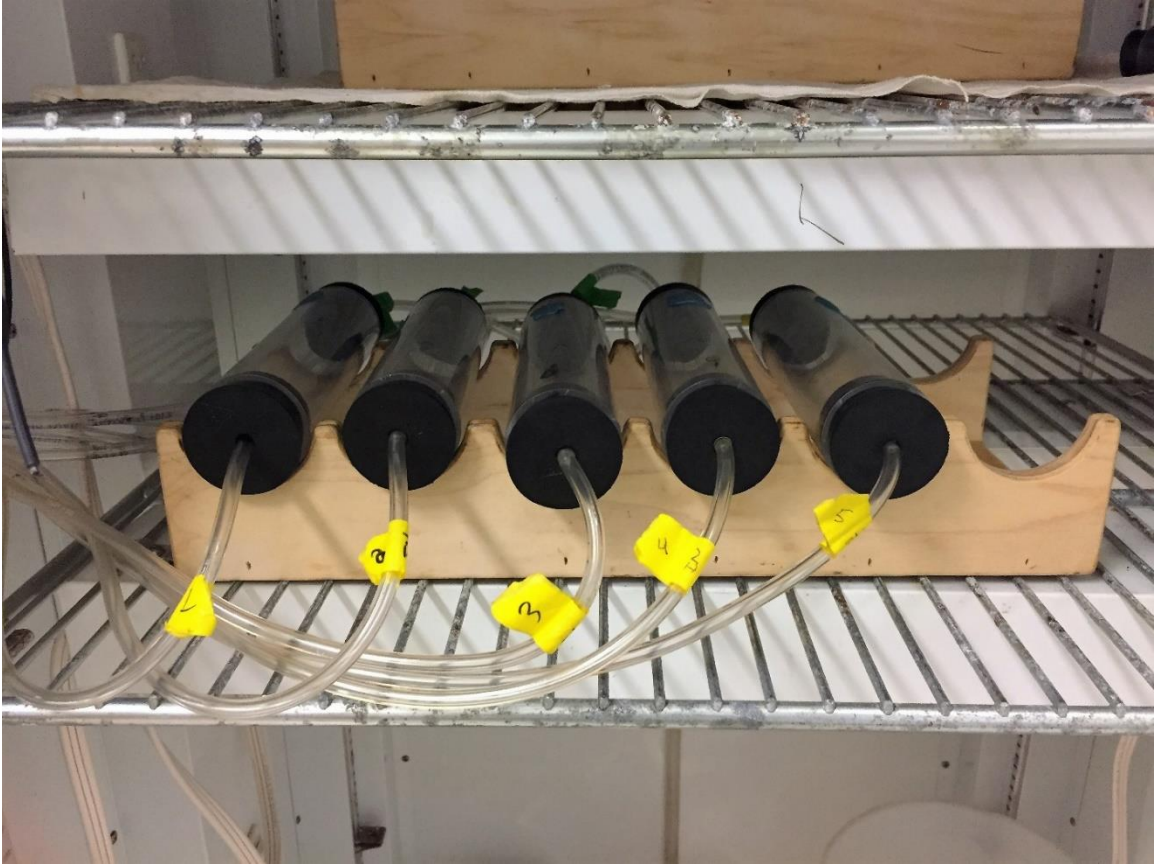
*Photo showing the sample chambers in the Percival cabinet while connected to the respiration system. The wooden rack holding the chambers was designed and constructed by Scientific Technical Services at Western Washington University.
