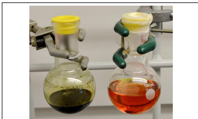
Figure 10. Comparison of non-decolorized (left) and decolorized (right) Isochrysis biodiesel fuels.
