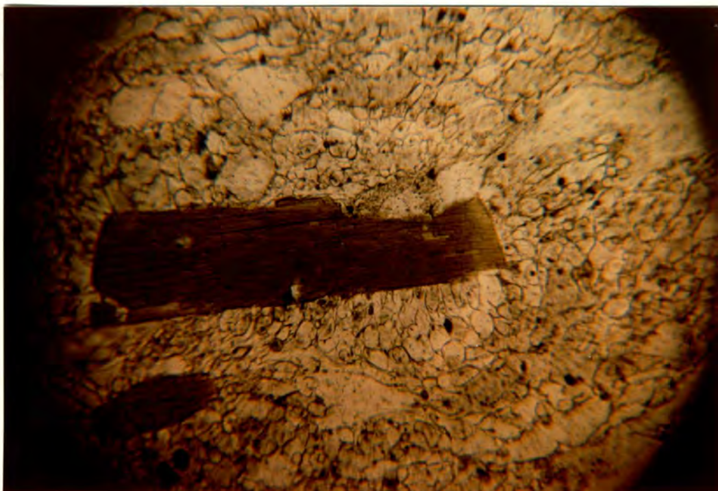
Figure 14. Photomicrographs of radial vesicle patterns, (a) Undisturbed radial vesicles, (b) Disturbed radial vesicles.
