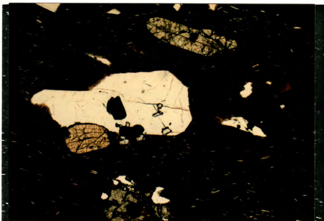
Figure 34. Phenocrysts in the dacite dike, sample 62. Plagioclase (white) contains magnetite and apatite inclusions. Clinopyroxene (top and in contact with plagioclase) is pale yellowish green. Brown hornblende is at right and olivine is at bottom. Plane light. Field of view 3 x 2 mm.
