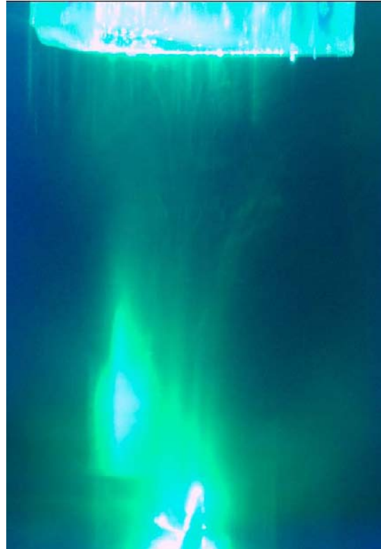
Figure 3-6: Long exposure time photography of the ionization region and portion of the drift region below the focusing tube.
