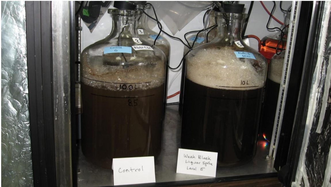
Figure 6. West Coast Regional Center laboratory biotreatment of Mill A simulated effluent samples. The reactor on the left contains only aerated stabilization basin influent and aerated stabilization basin treatment pond wastewater (reactor control), and the reactor on the right contains aerated stabilization basin influent, aerated stabilization basin treatment pond wastewater, and the highest spike level of weak black liquor (WBL spike 5).
