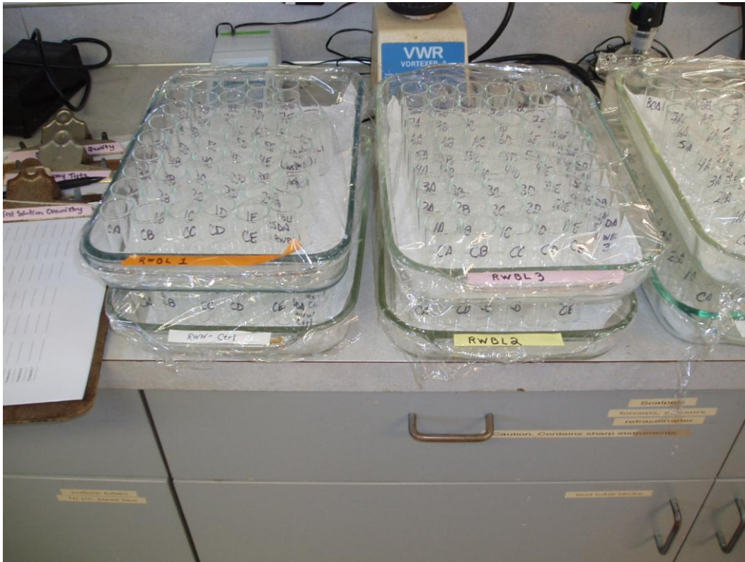
Figure 9. Test chambers for Mytilus galloprovincialis 48-h embryo-larval development toxicity tests.
