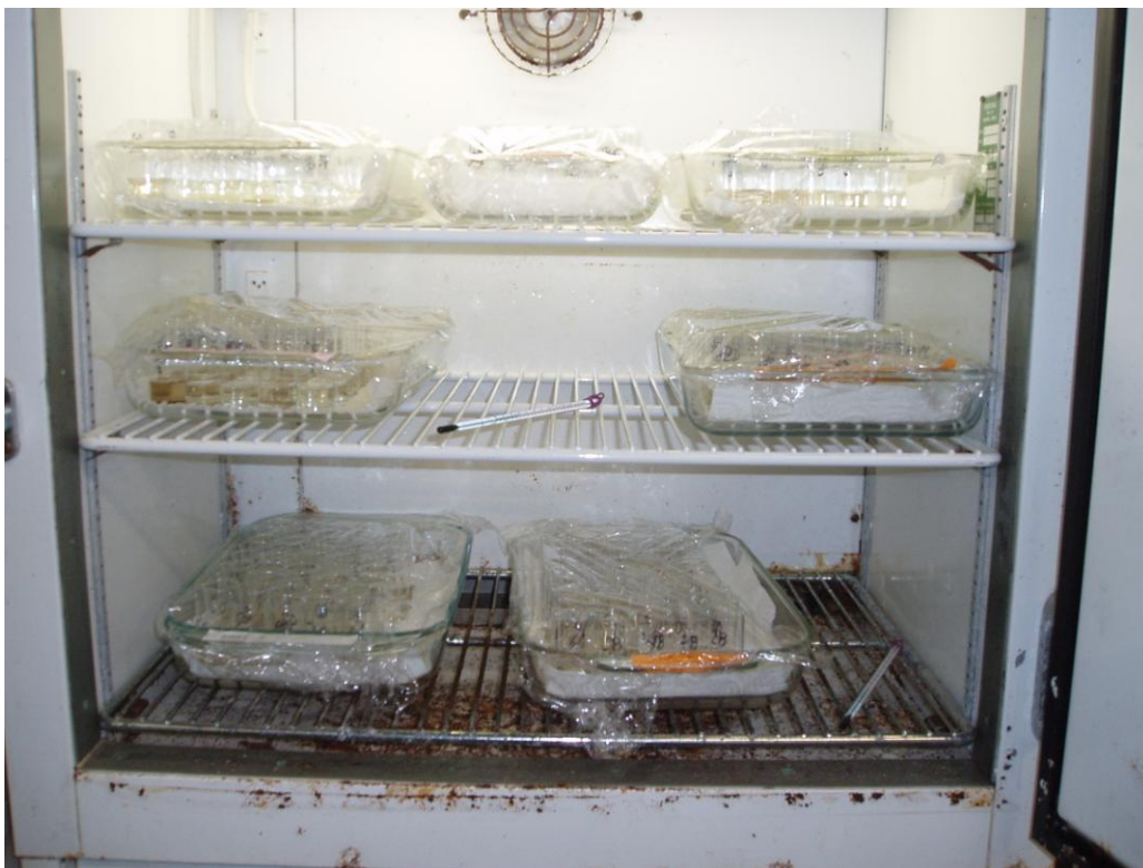
Figure 12. Environmental chamber at initiation of 48-h Mytilus galloprovincialis test.
