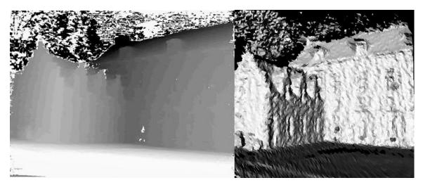
Figure 6: The disparity map (left) and reconstructed scene (right)
