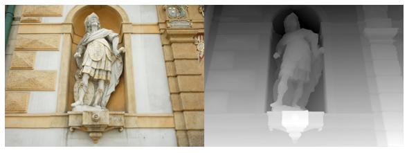
Figure 5: The reference image (left) and obtained disparity map (right)
