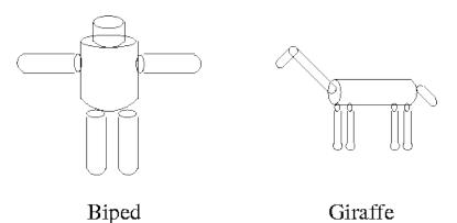
Figure 8: Constructive Solid Geometry (CSG) representation of objects
