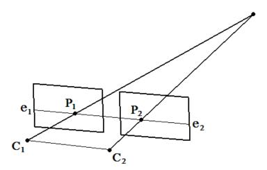
Figure 4: Epipolar geometry used to calculate the depth of a projected pixel.  $C_1$  and  $C_2$  represent the left and right cameras, while  $e_1$  and  $e_2$  represent the epipolar line, and  $P_1$   $P_2$  are the projected coordinates in the image.
