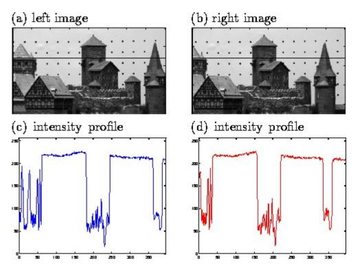
*Figure 2: An intensity profile is developed for each image using the coloration intensity from each pixel*
