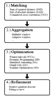
Figure 1: The steps of stereo correspondence algorithms
