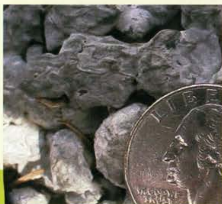
A quarter shows the large gravel used to produce porous concrete. photo by Chris Phillips
