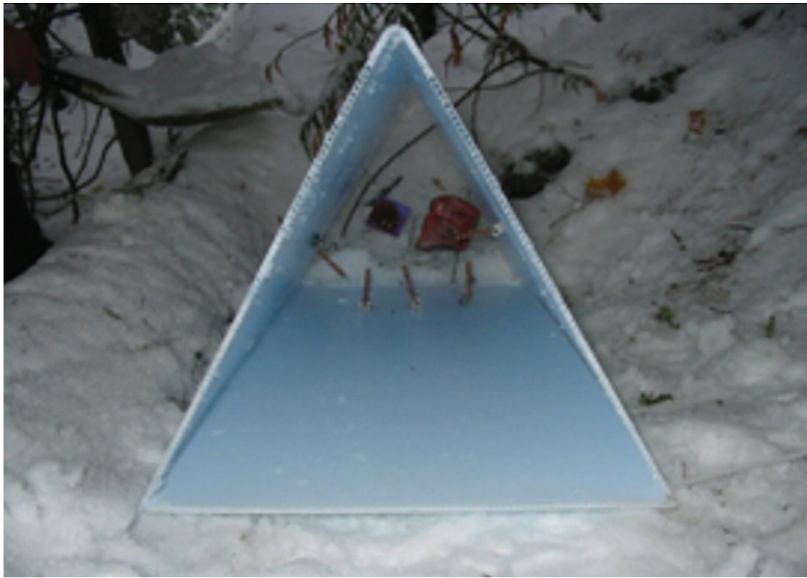
Figure 2. Non-invasive hair snare station with five gun brushes, bait, and mesh wire at back to create a one-way opening.
