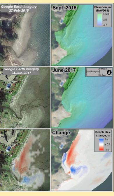
Four sub-regional areas within the drift cell had significant morphology change between the two surveys: the restoration site, a stream outlet (shown above), an accretionary beach with sand wave migration, and Hunter Point. The rest of the drift cell remained relatively unchanged. The figure to the right shows these changes and presents a preliminary sediment budget for the drift cell.
