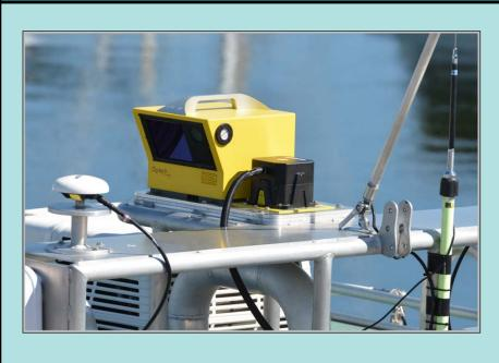
Boat-based topographic lidar surveys were conducted in Sept. 2015, about a year before removal of the shoreline armor, and June 2017, almost eight months following removal. Each survey involved the collection of boat-based lidar along 5 km of shoreline using Real Time
