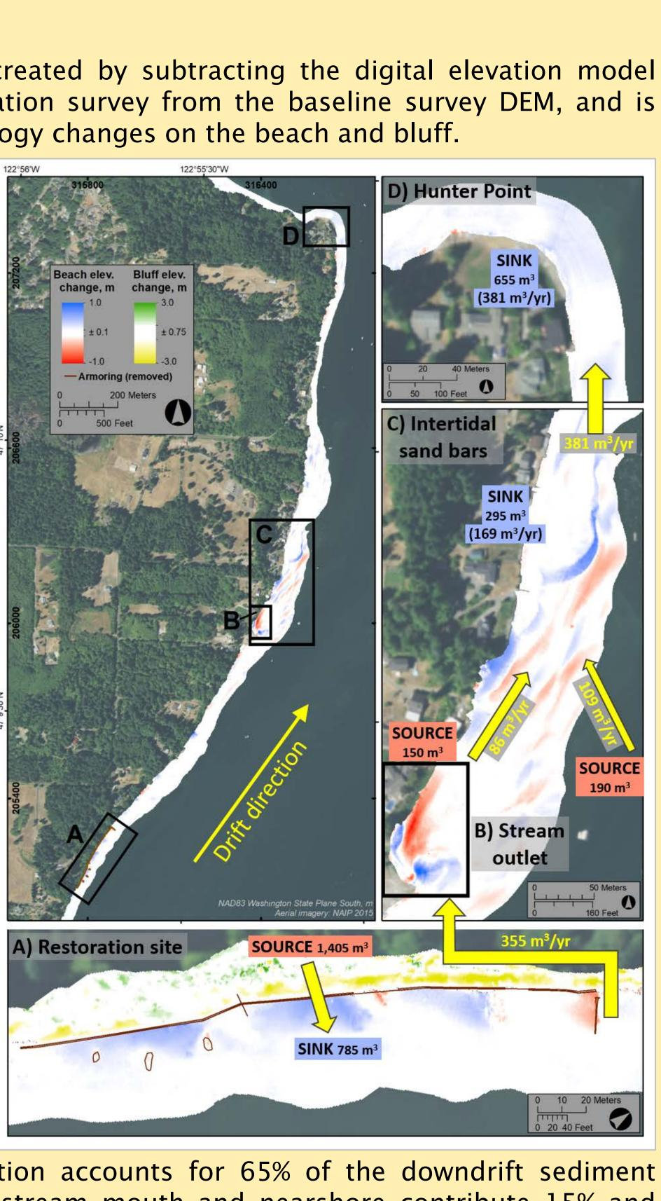
The feeder bluff restoration accounts for 65% of the downdrift sediment accumulation, while the stream mouth and nearshore contribute 15% and 20%, respectively.
