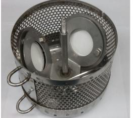
Jpper Support ring pper membrane disl wer membrane disl ower support ring
