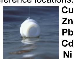
POCIS<sup>3</sup> sample weakly hydrophobic (log K<sub>ow</sub> ≤4) organic chemicals that bind to a polymeric (hydrophiliclipophilic-balanced; HLB) sorbent sandwiched between polyethersoulfone (PES) membranes.
