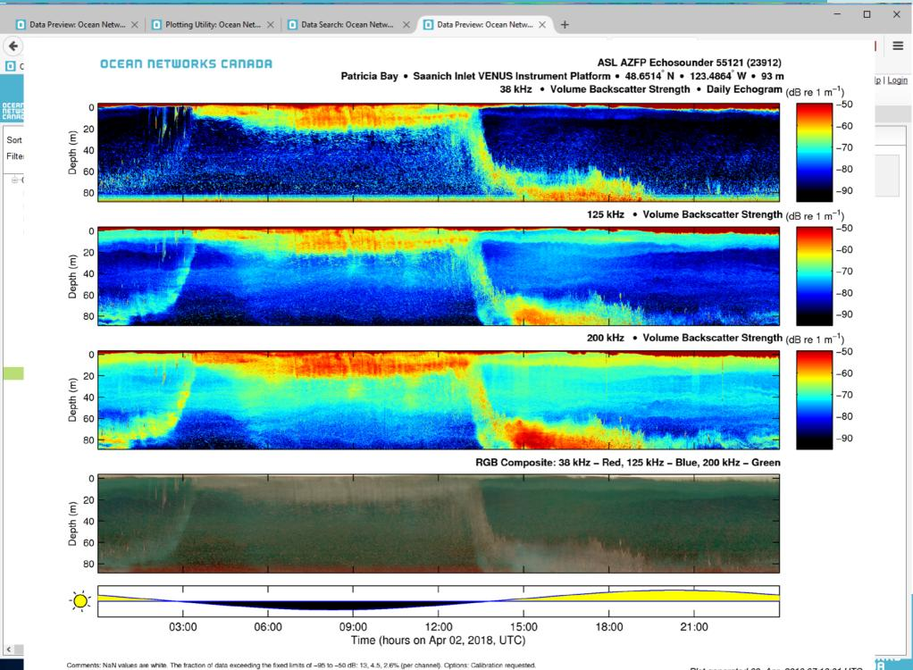
Comments: NaN values are white. The fraction of data exceeding the fixed limits of -95 to -50 dB: 13, 4.5, 2.6% (per channel). Options: Calibration requested Ensemble period: 29.3 sec.
