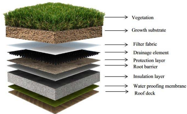
Figure 4: Construction of green roof (Kapsalaki, 2017)
