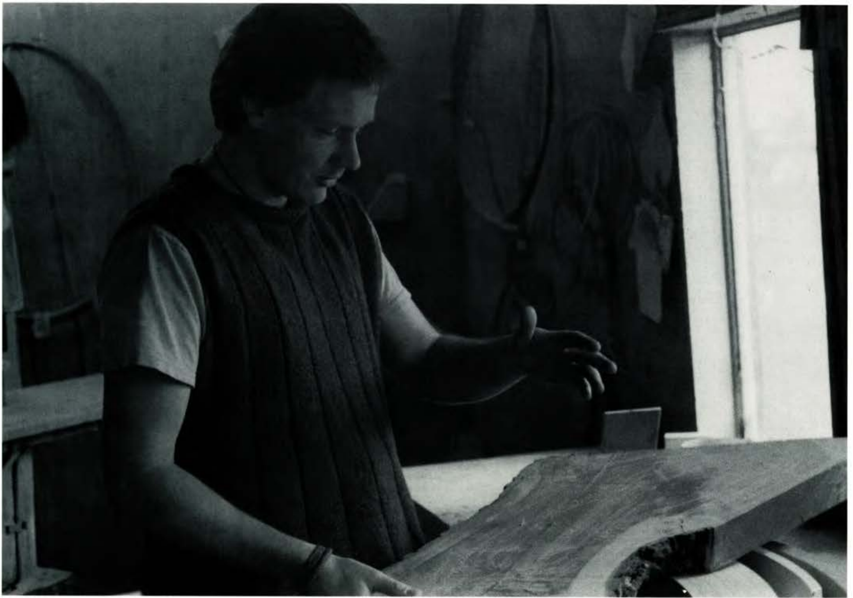
Degan hefts a slab of prized applewood onto his workbench to cut into staves. They then will be glued together into a conga drum.
