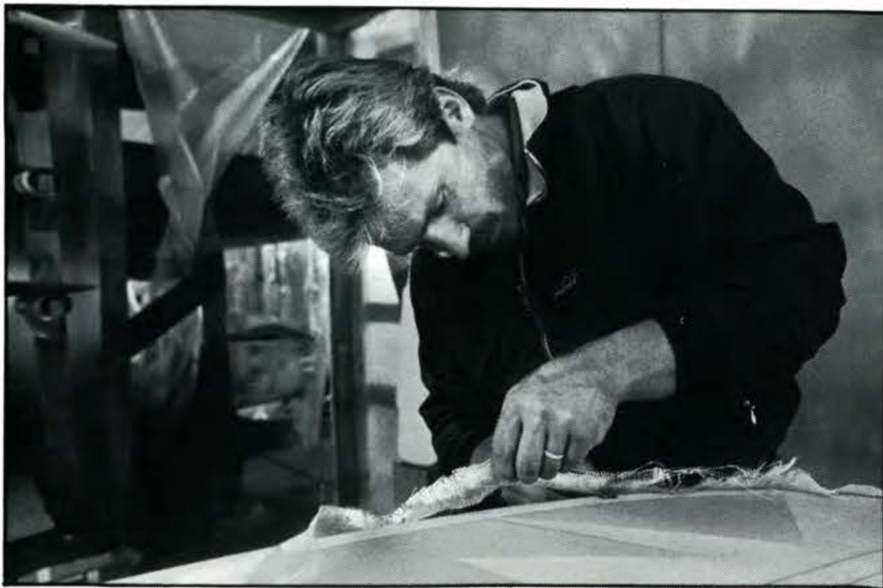
Derek Hilleary trims excess resin and fiberglass from one of his sailboards.
