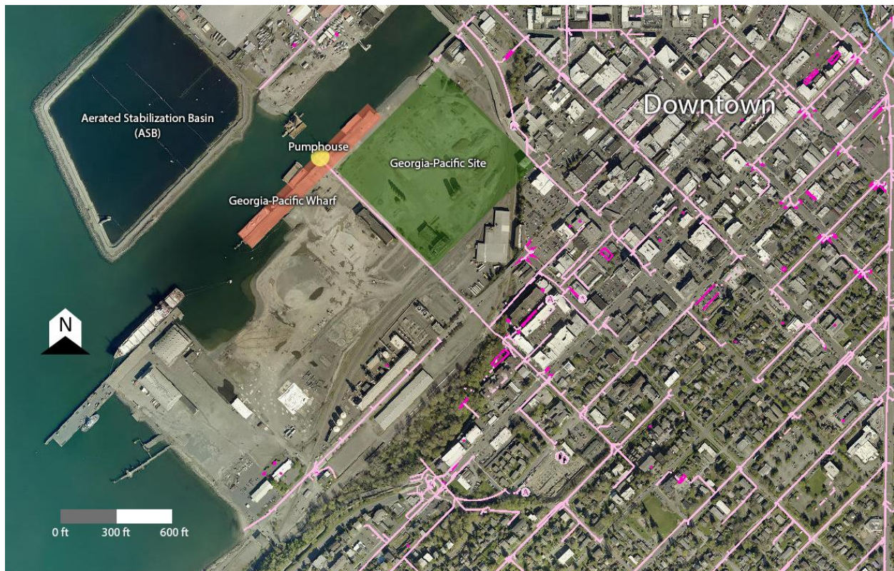
Figure 18: Current storm water lines (pink) to pumphouse from downtown and GP site (green) and wharf (orange) (City of Bellingham, 2017).
