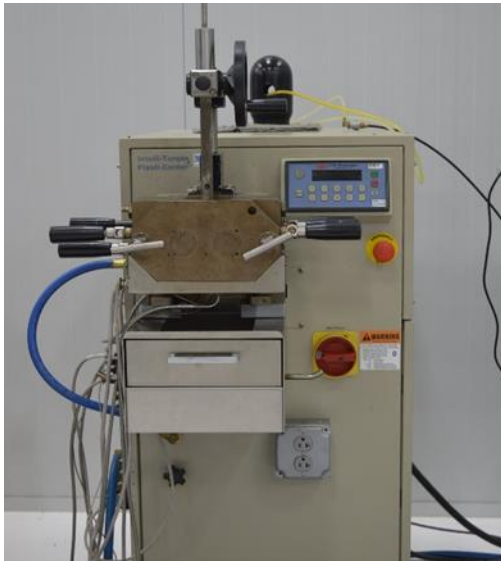
Figure 8. The above figure is a picture of the Brabender mixer that was used to identify promising TPV formulations.
