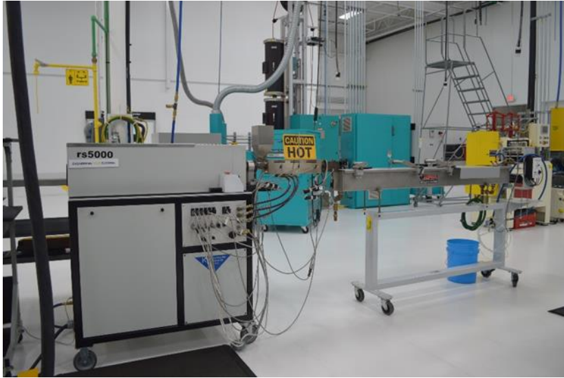
Figure 10. The above figure is a picture of the single screw extruder tape extrusion line that was used to make tape extrusion samples for tensile testing and other material characterization.
