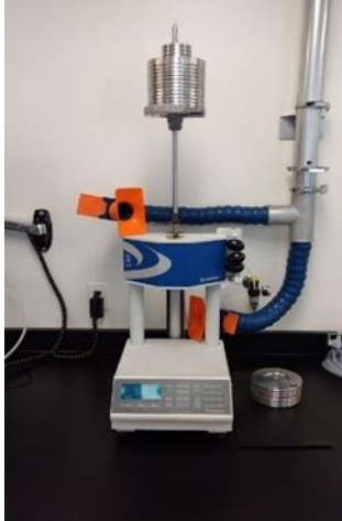
Figure 12. The above figure is a picture of the Melt Flow Indexer that was to determine the flow rate of TPV samples at 230°C. These flowrates served as general viscosity measurements and helped determine TPV processability.
