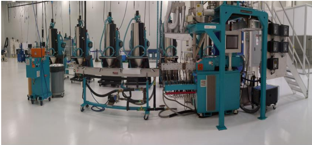
Figure 9. The above figure is a picture of the 26 mm fully intermeshing, co-rotating twin-screw extruder, water bath, and rubber pelletizer that was used to determine the ideal amount of curative and cure system for TPV samples.
