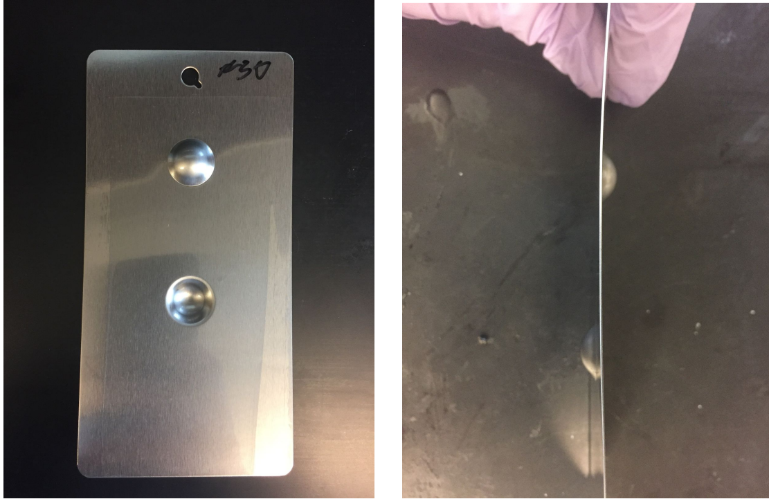
Figure 26: Images of an E30 coated panel subjected to forward and reverse impact testing.
