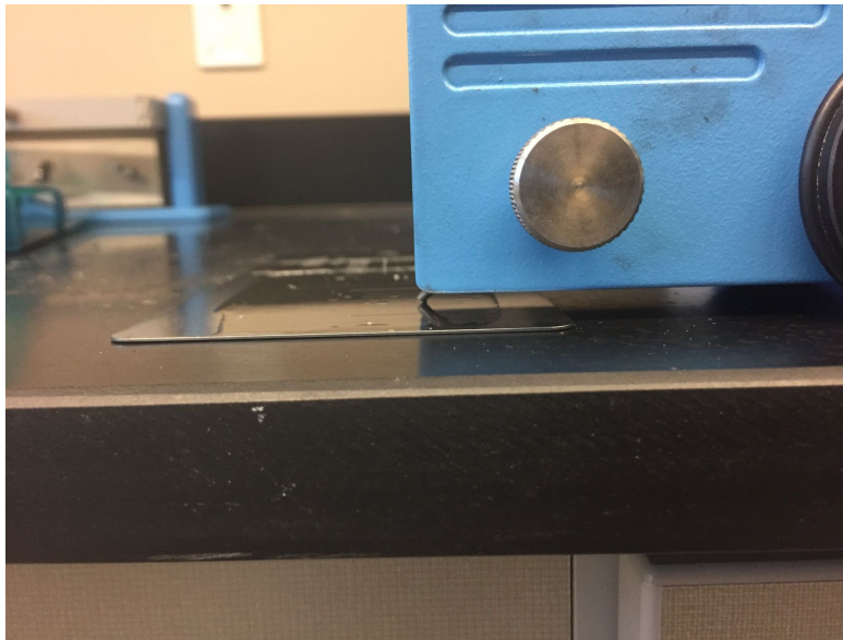
Figure 22: Side view of pencil hardness tester during test.
