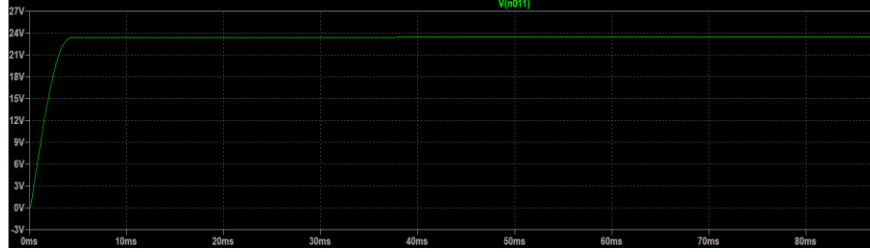
Figure 32: Output of the AC/DC Rectifier
