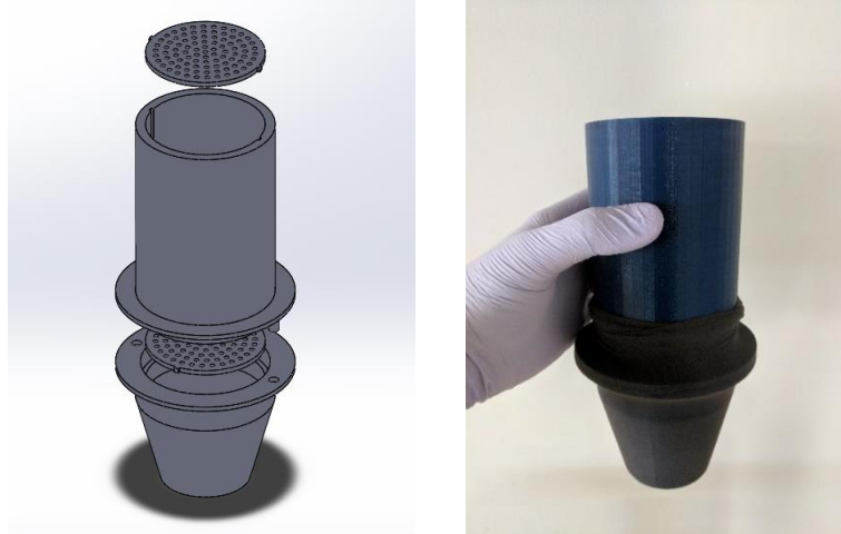
Figure 4: The testing apparatus designed for this study. a - The model in SolidWorks. b - The 3D printed fully assembled apparatus.
