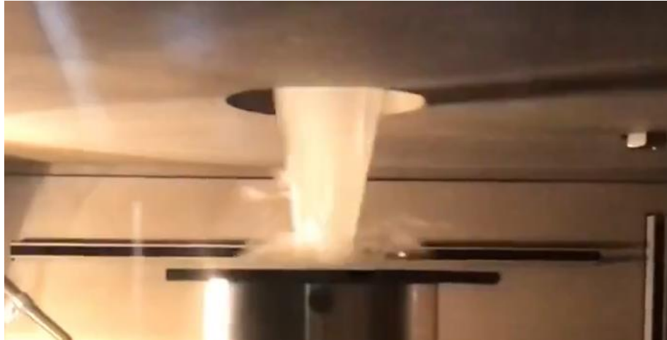
Figure 21. Moment of impact, finalized impactor, 6 J.
