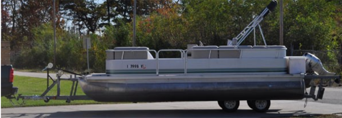
Figure 1. Center lift trailer with a small frame compared to the large pontoon boat.
