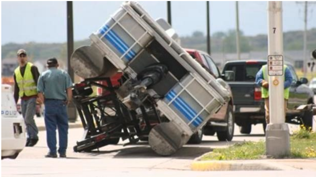
Figure 2. Accidents resulting from sharp turns with a center lift trailer.
