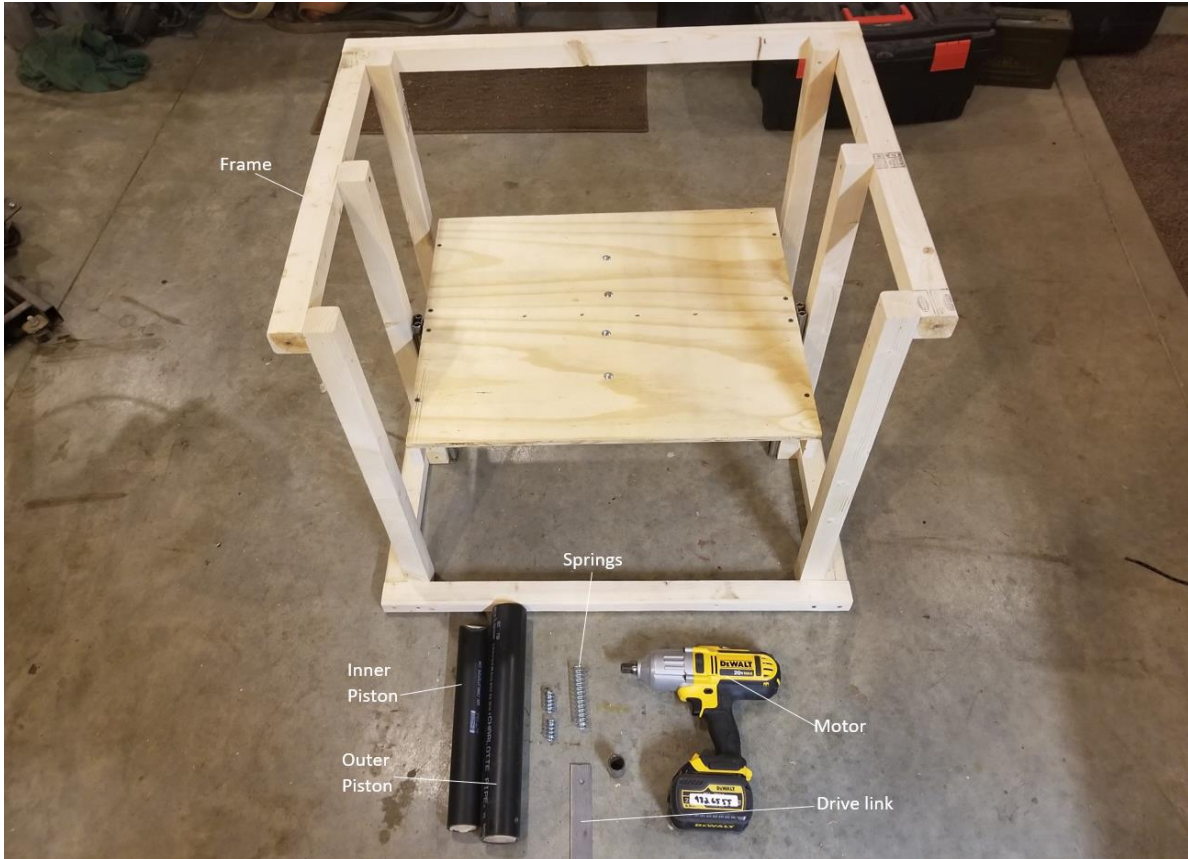
Figure 4: Components of the rotating lever arm design for raising the target platform
