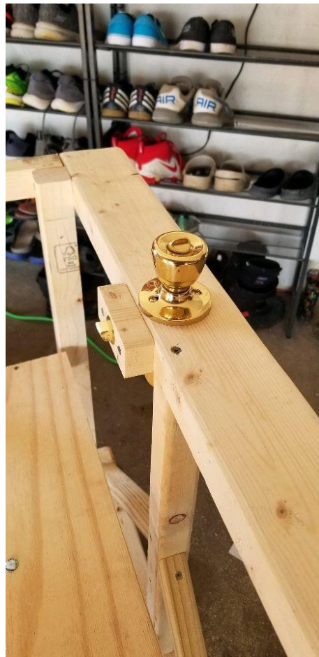
Figure 9: The door knob assembly mounted onto the frame which latches the platform in its starting position and releases the target when a signal is received from the Arduino
