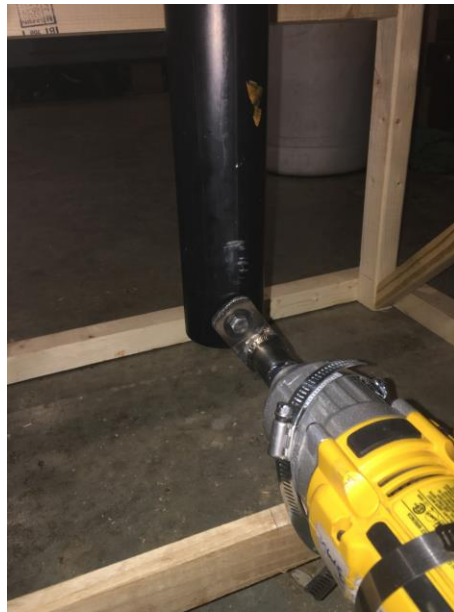
Figure 5: Linkage system to raise the target system with impact wrench
