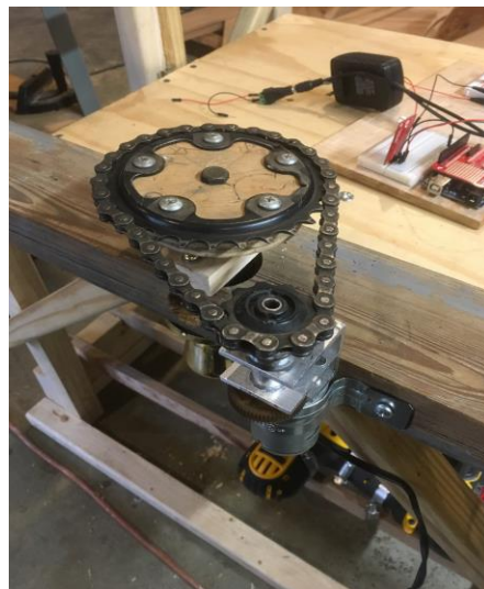
Figure 11: Intermediate design with sprocket torque multiplier of only 2.8 and overall torque multiplier of 11.2 (Unsuccessful design)
