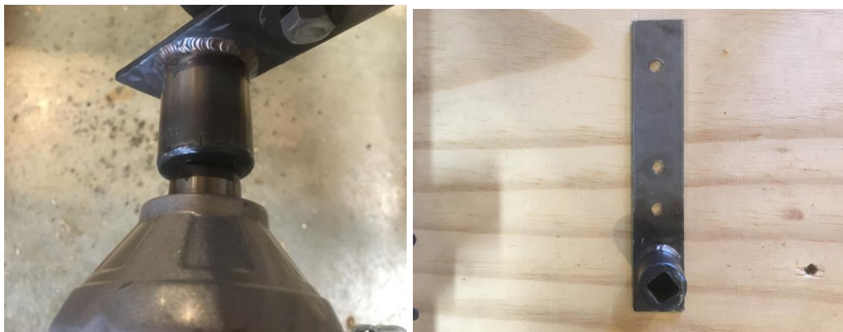
Figure 7: 1/2" Socket correctly mounted onto the 1/2" Impact Wrench drive shaft.
