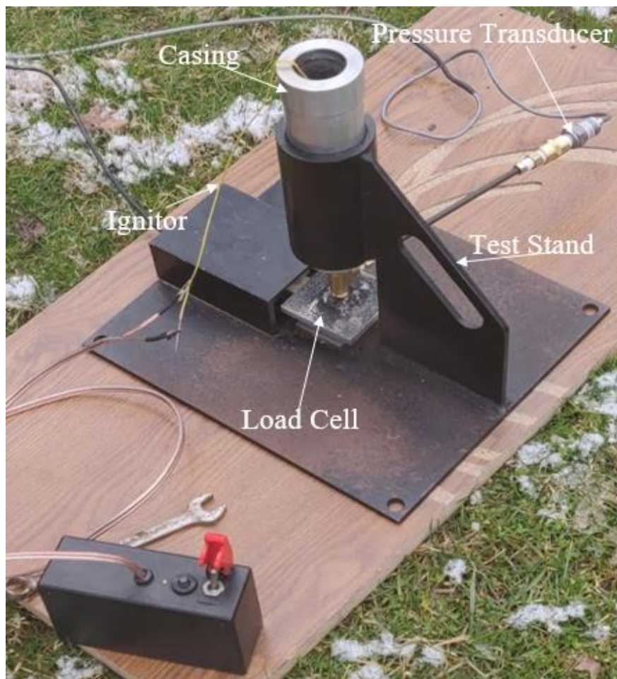
Figure 4 - Static test stand used for each burn test with equipment components indicated
