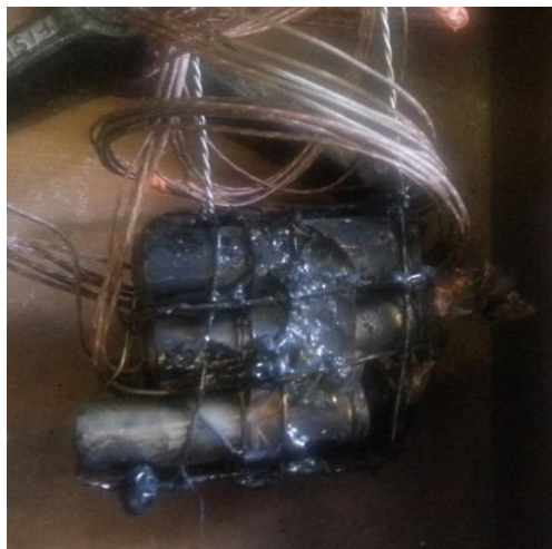
Figure 9: Photo of a battery pack after the completion of the experiment.
