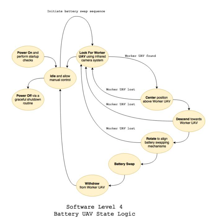
Figure 21 – Battery UAV State Machine [ND]
