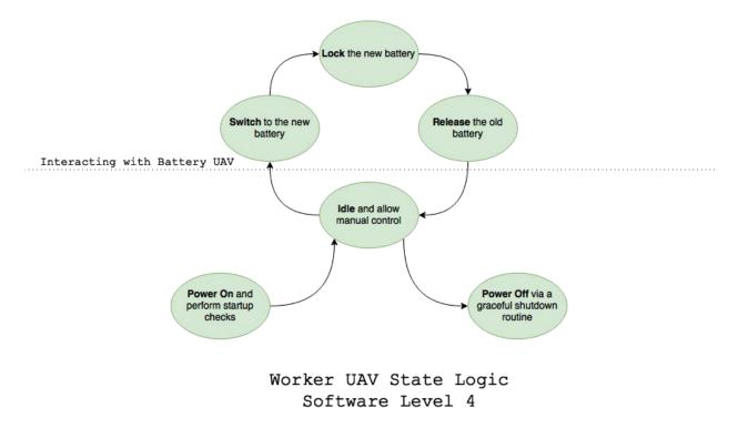
Figure 23 – Worker UAV State Machine [ND]
