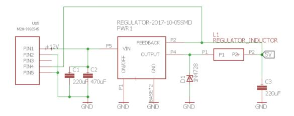
Figure 14 – Voltage Regulator [WG]
