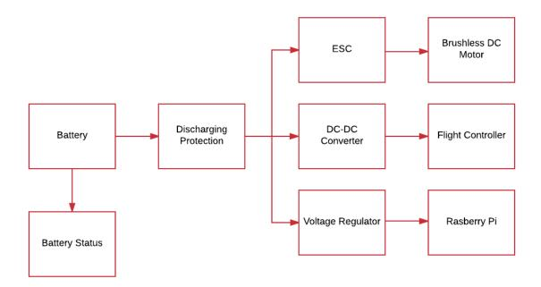
Figure 06 - Power Management System Level 1 Block Diagram
