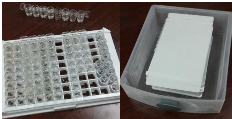
Figure 5 and 6: Left, the trays that the SRT hydrogels were created and stored in. These were detachable which made testing easier. Right, the hydrogel trays were placed in a container whose bottom was covered with water to help keep the gels hydrated. Despite efforts to keep the gels hydrated, the gels still dried out, causing difficulties in comparing tests.
